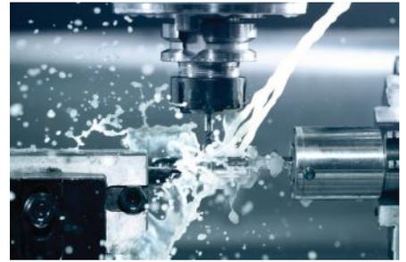
loss via the metal cuttings, and so the levels need to be refilled with the correct mixture ratio—this is where proportional dosing systems come into play.
