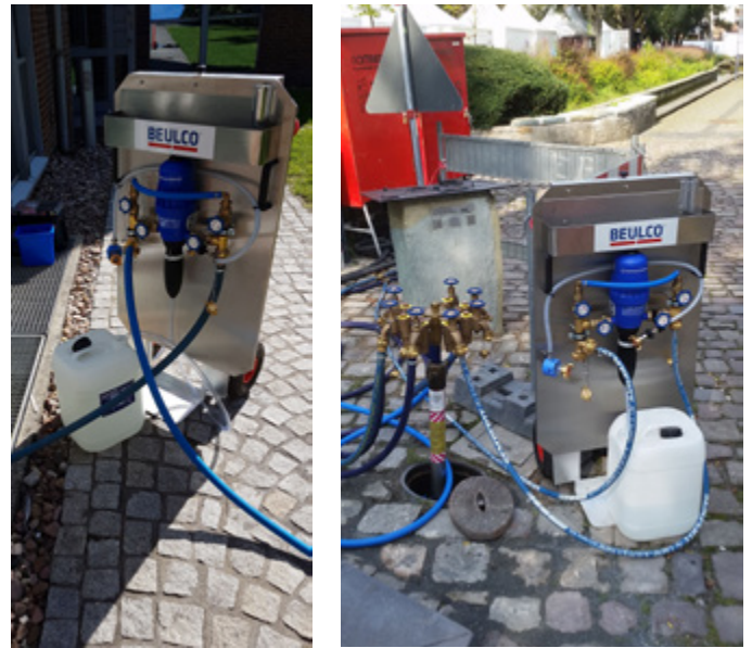
Figure 2: Mobile cleaning and disinfecting system
