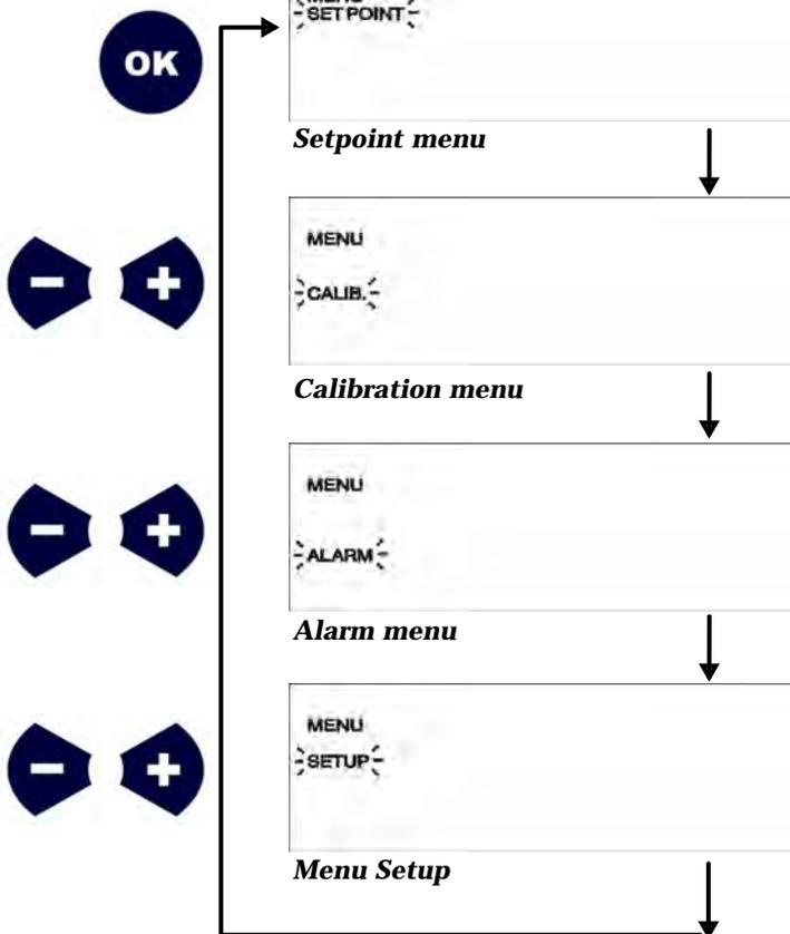
To enter in **SETUP** menu scroll all menus with + and - buttons up to reach the desired menu (on display will show **SETUP**), press **OK** to confirm.
