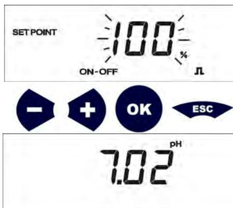
Only in ON/OFF mode is it possible to define the time delay with regards to the Setpoint start-up, press the + and - keys to set the time in minutes and seconds. Press the **OK** key to confirm the values.
