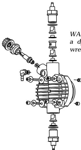
WARNING: to tightening the four screws, use a dynamometric screw driver, set the torque wrench to 1,8N x m.
