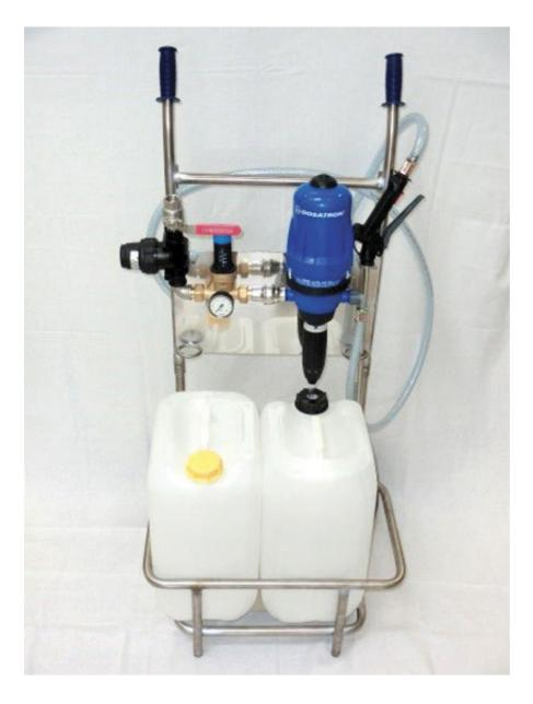
Mobile dosing equipment on a trolley
