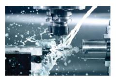
loss via the metal cuttings, and so the levels need be refilled with the correct mixture ratio—this is where proportional dosing systems come into play.
