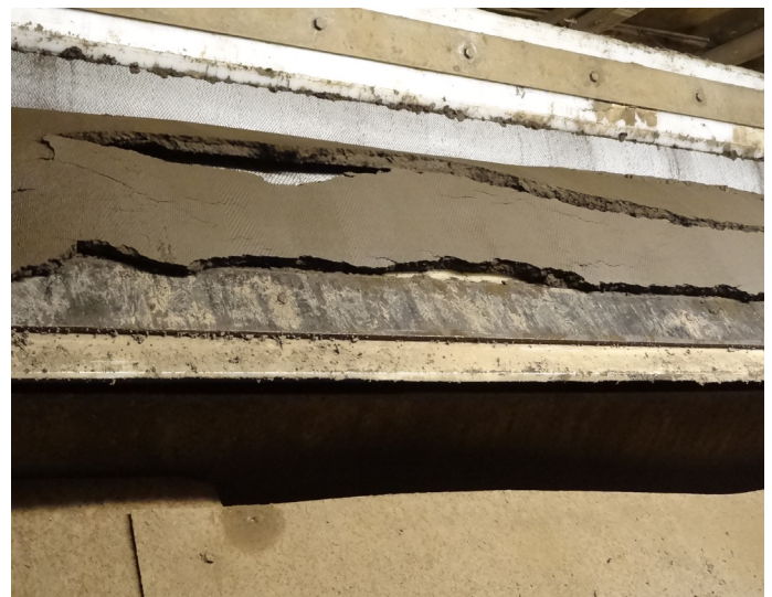
Filter cake nearly dry after leaving the belt filter.
